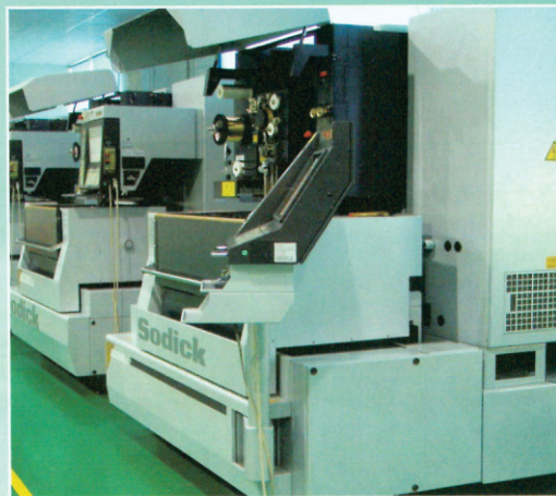
Sodick low-speed wire cutting machine Mould production
